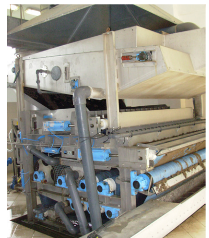
View of the filter press currently used at the Mytilene STP
